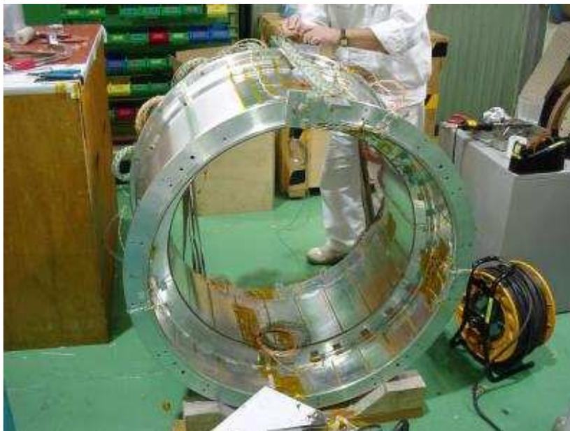
Figure 11: The central part of the COBRA magnet which contains the central coil, two gradient coils, and an aluminum support structure.
