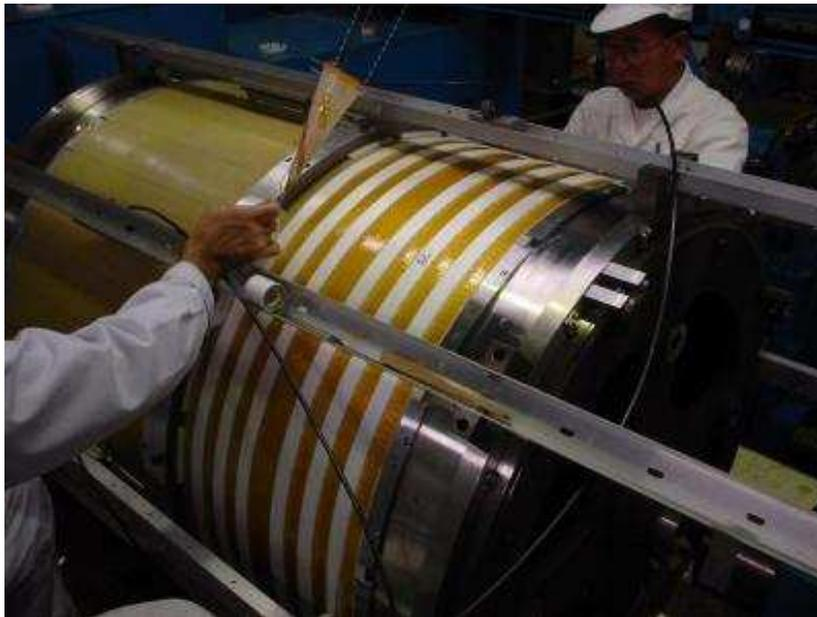
Figure 19: The winding of the end coil where a block winding technique is employed.
