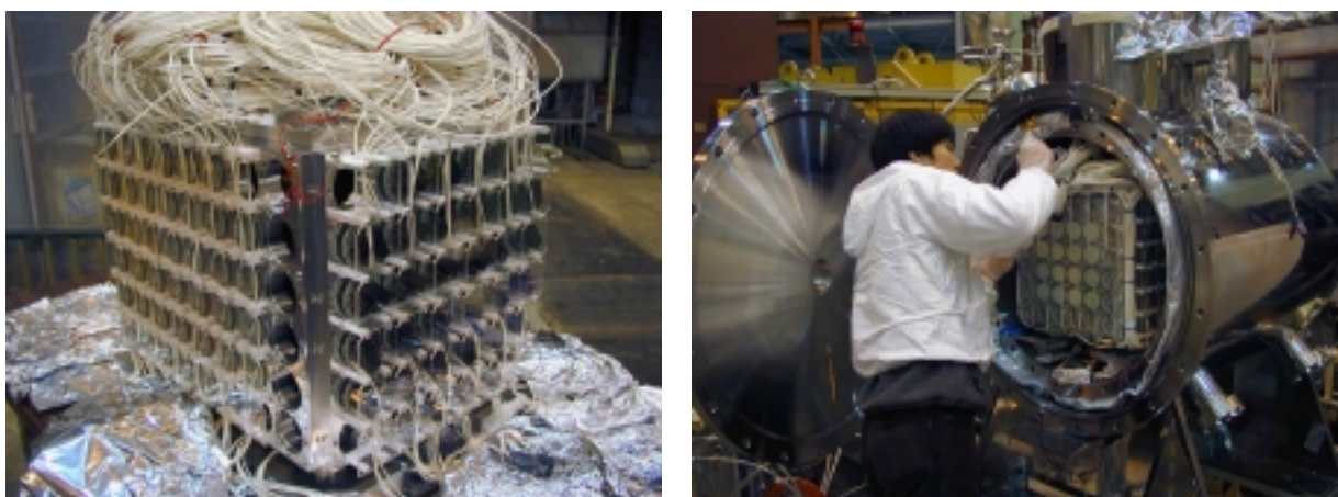
Fig. 12 PMTs assembled in a rectangular shape (left). The PMTs are installed in the cooling vessel (right).
