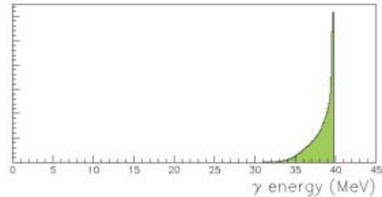
calculated  $\gamma$  beam energy spectrum at TERAS
