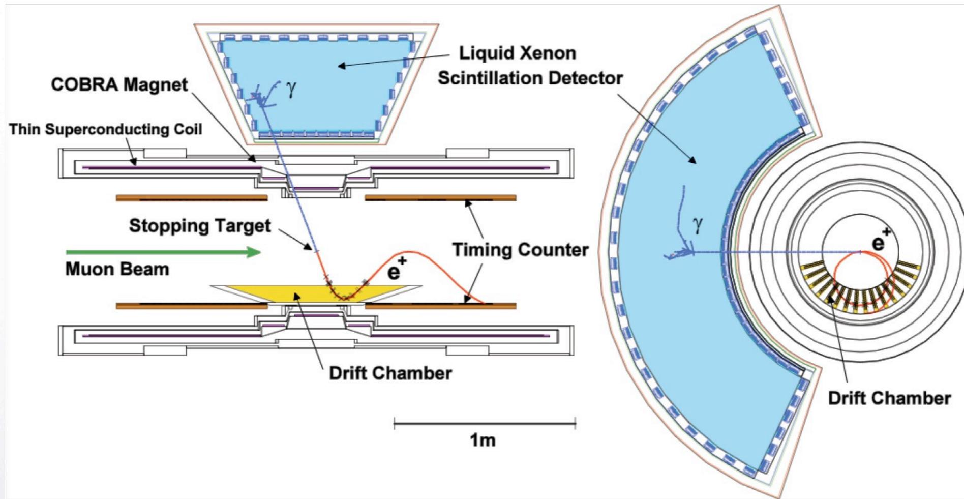
Liquid xenon gamma ray detector
