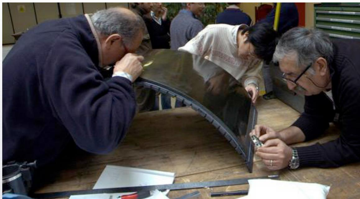
Honeycomb window with carbon fiber plates
