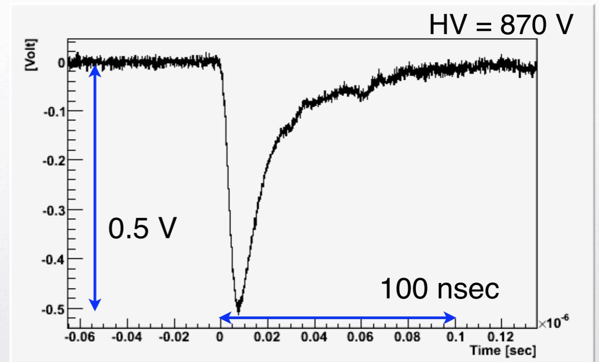
PMT signal by 17.6 MeV gamma ray from  $\text{Li}(p,\gamma)\text{Be}$
