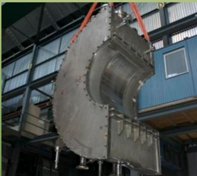
Liquid Xenon Scintillation Detector for gamma-ray
