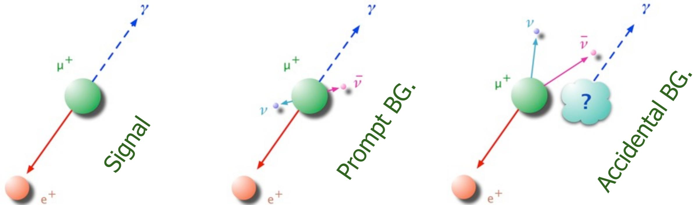
❖ Clear 2-body kinematics ( $E_e = E_\gamma = 52.8 \text{ MeV}$ ,  $\theta_{e\gamma} = 180^\circ$ , Time Coincidence)
