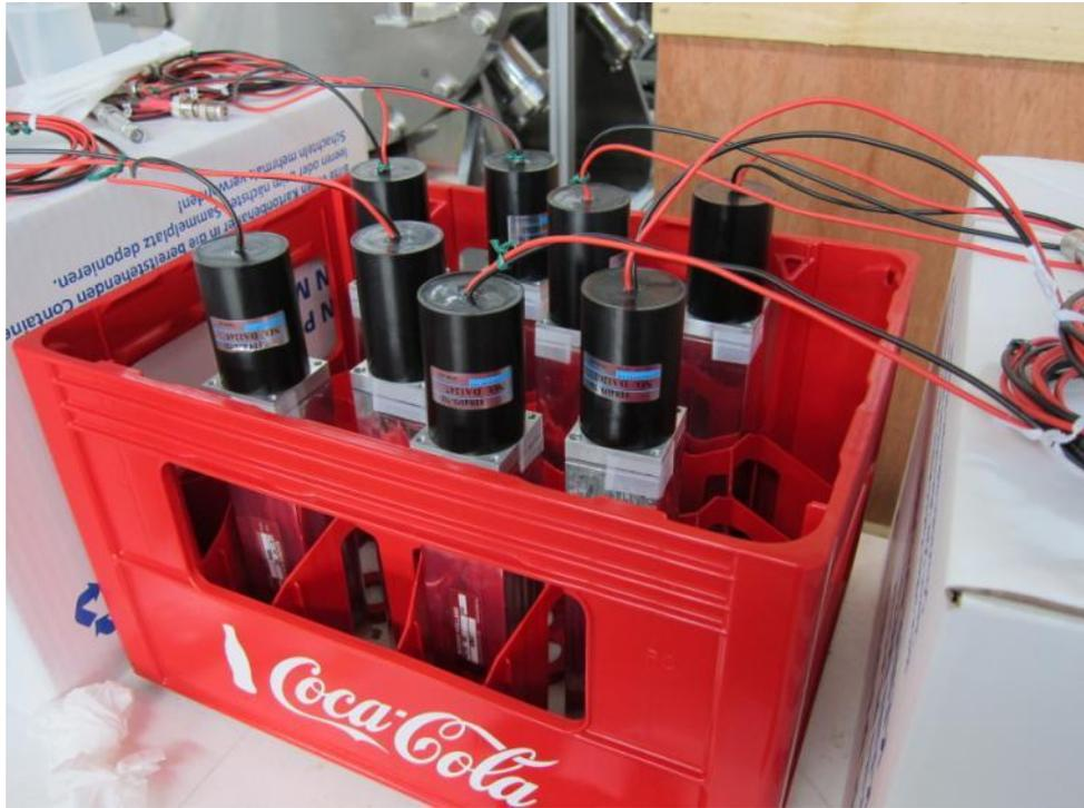
← BGO & PMT were hold until cement cured in case
