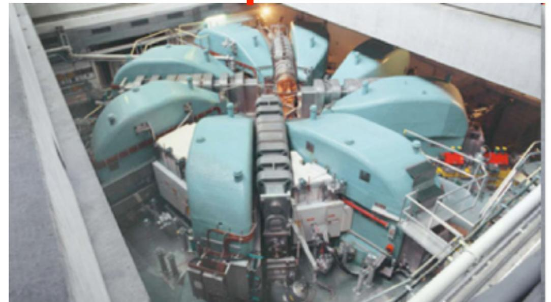
1.3MW high intensity proton accelerator
