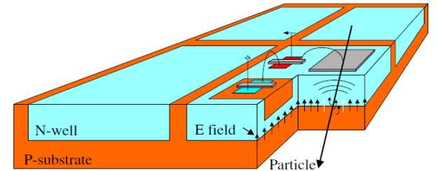
(High voltage monolithic active pixel sensors)
