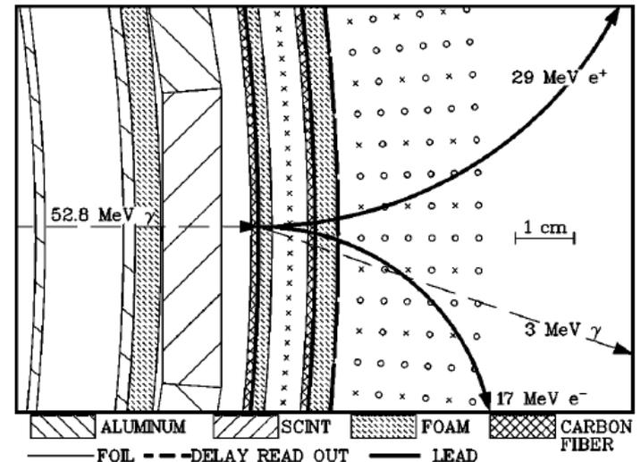
FIG. 5. A cross section of a pair spectrometer layer, showing the aluminum support cylinder for an inner layer, and the timing scintillators, conversion cylinders, MWPC and drift detectors for the next outer layer. A typical conversion in the first conversion cylinder is shown.
