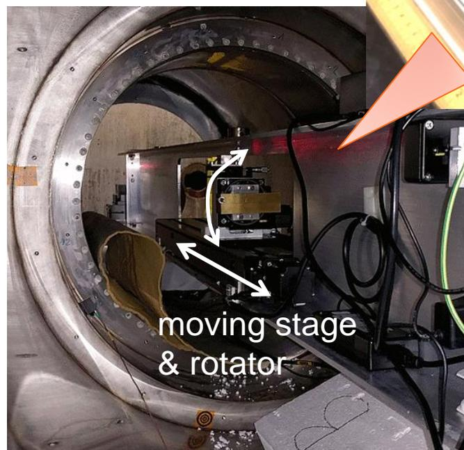
Position of the stage is measured by laser and monitored by laser and bubble level + camera.
