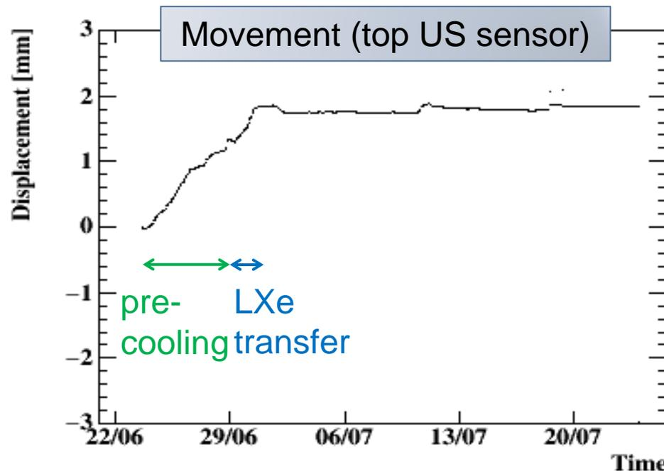
Moved mostly during the pre-cooling due to heat shrink. Result was roughly consistent with what we expect ( $\sim 1.6 \times 10^{-3} \text{ mm/m/K}$  heat shrink to bottom direction)
