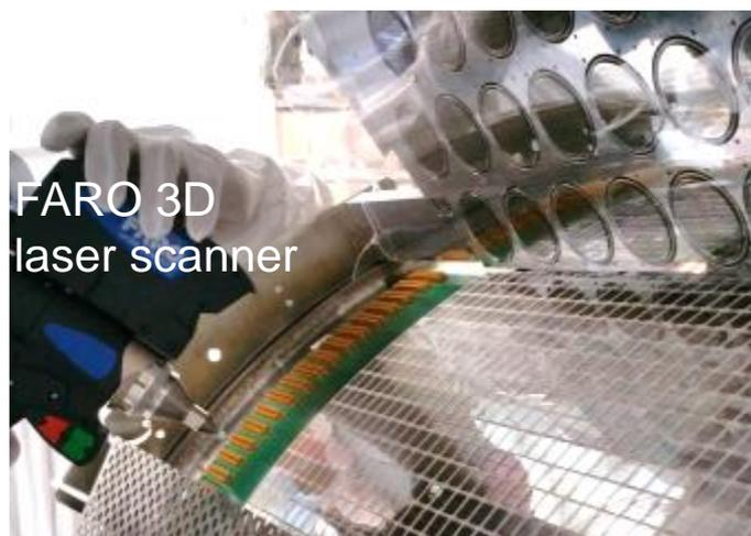
However, inner cryostat deforms by heat shrink and LXe load.
