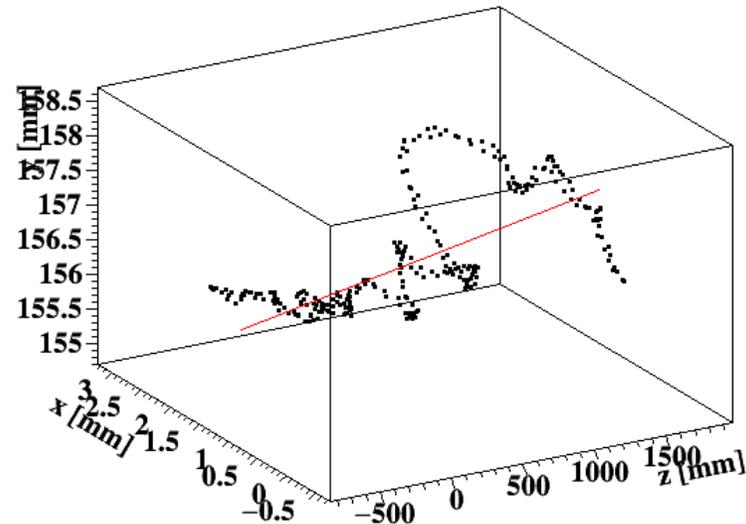
After the corrections of tilt and Z linearity, deviation (RMS) of surveyed X,Y,Z positions from calculated position were  $\sim 200$   $\mu\text{m}$  in X,Y,  $\sim 30$   $\mu\text{m}$  in Z.
