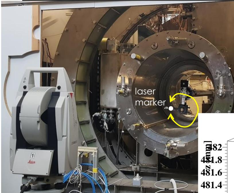
Position and tilt of the arms are measured in laser survey.
