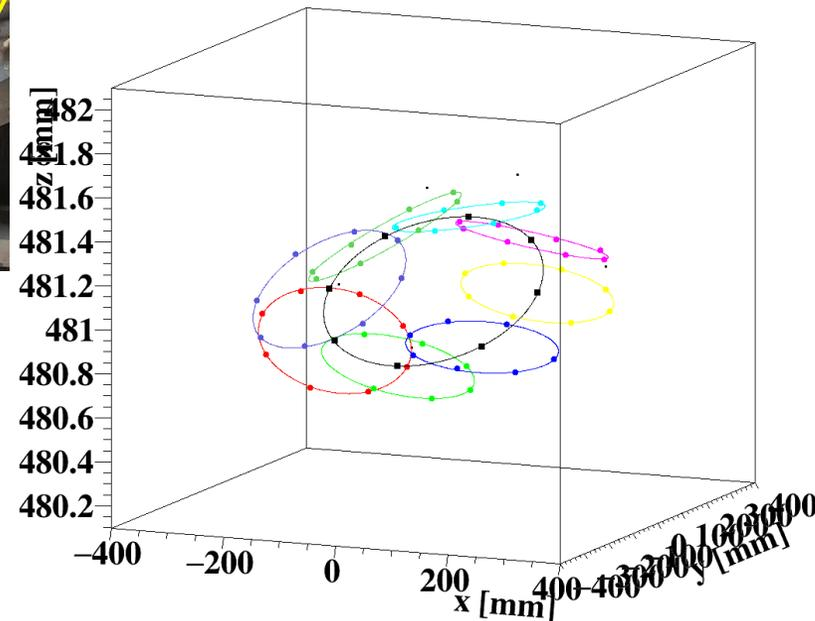
Z position is found to vary by  $\sim 0.5$ mm due to tilt, but we can correct this based on the tilt parameters obtained in this survey.
