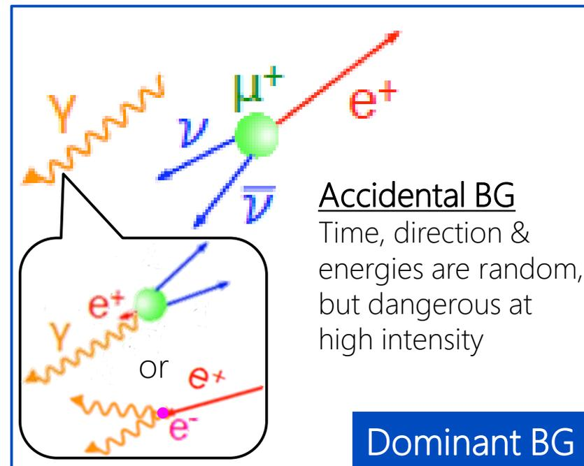
$$R_{BG} \propto R_{\mu}^2 \cdot \delta E_e \cdot (\delta E_{\gamma})^2 \cdot \delta\omega/4\pi \cdot \delta t$$
