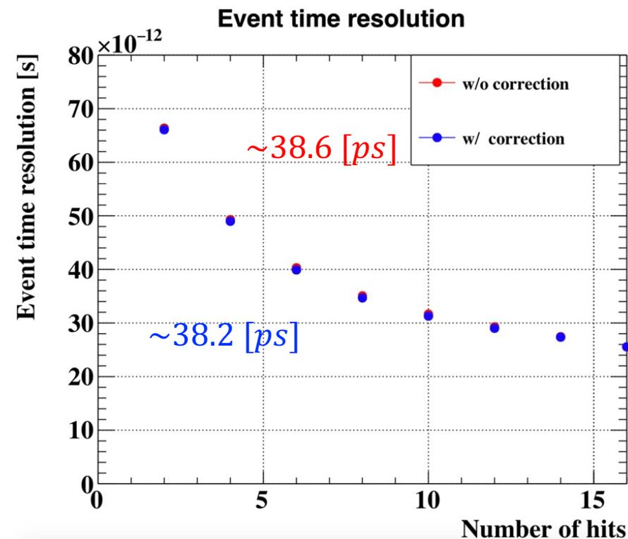
pTC resolution using even-odd analysis on 2017 data
