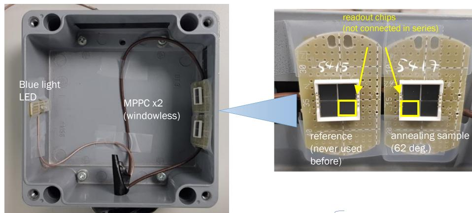
Measurements were done before/after annealing. In light tight box (not in thermal chamber), clean room.
