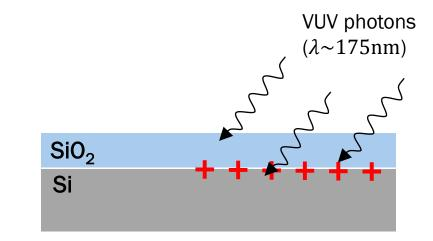
Accumulation of holes near SiO<sub>2</sub>-Si interface  $\rightarrow$  reduction of carrier collection efficiency Similar phenomena is known for UV photo diode.
