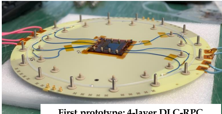
First prototype; 4-layer DLC-RPC (Reported at JPS2022 autumn, and JPS2023 spring)
