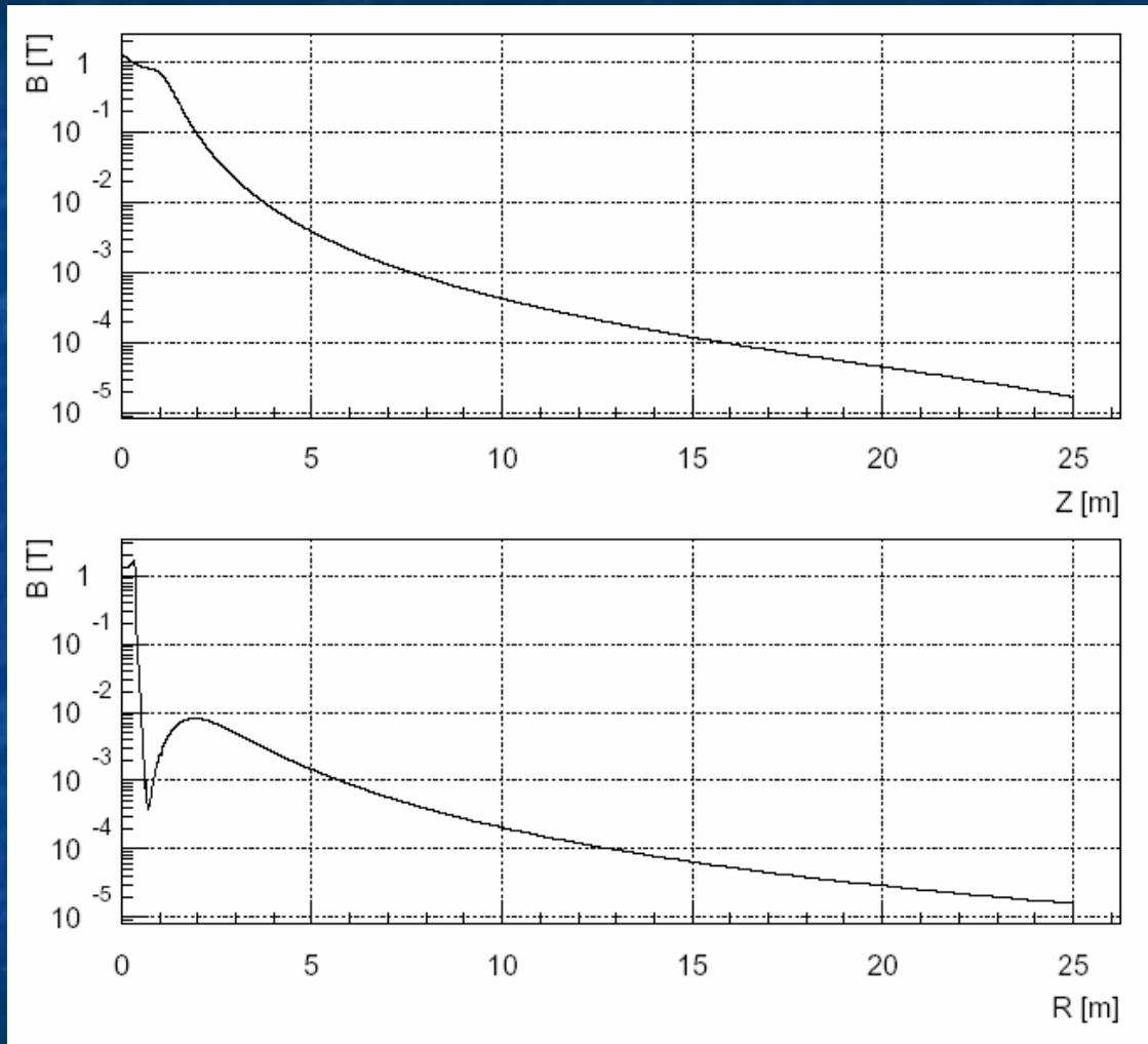
**~10 Gauss at 5-7m    ~1 Gauss at 12-15m**
