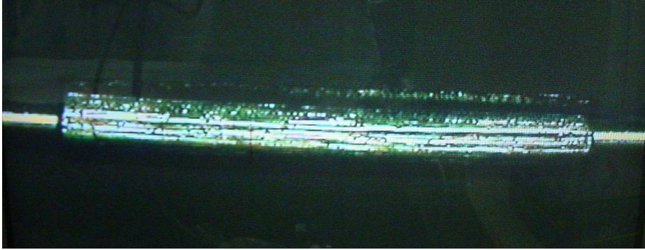
Figure 1: Micropicture of a Am-source mounted on a 100\ \mu\text{m} -diameter wire.
