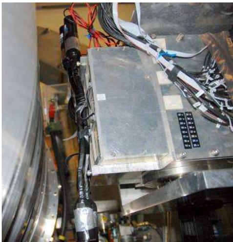
(a) The NaI calorimeter, consisting of a lead plate, plastic scintillating bars, and NaI crystals.
