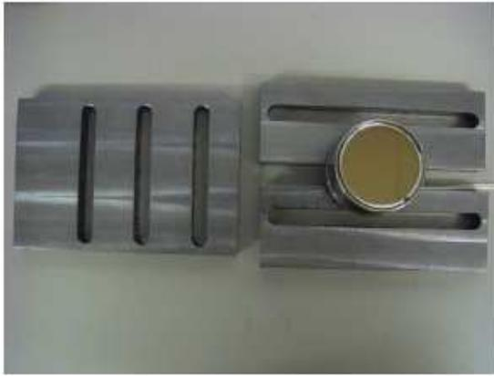
(a) Lead bricks with 1 cm wide slits. A PMT is shown for reference on top of the bricks on the right.
