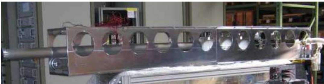
(b) The bellows system for insertion and extraction of the  $Li_2B_4O_7$  target.
