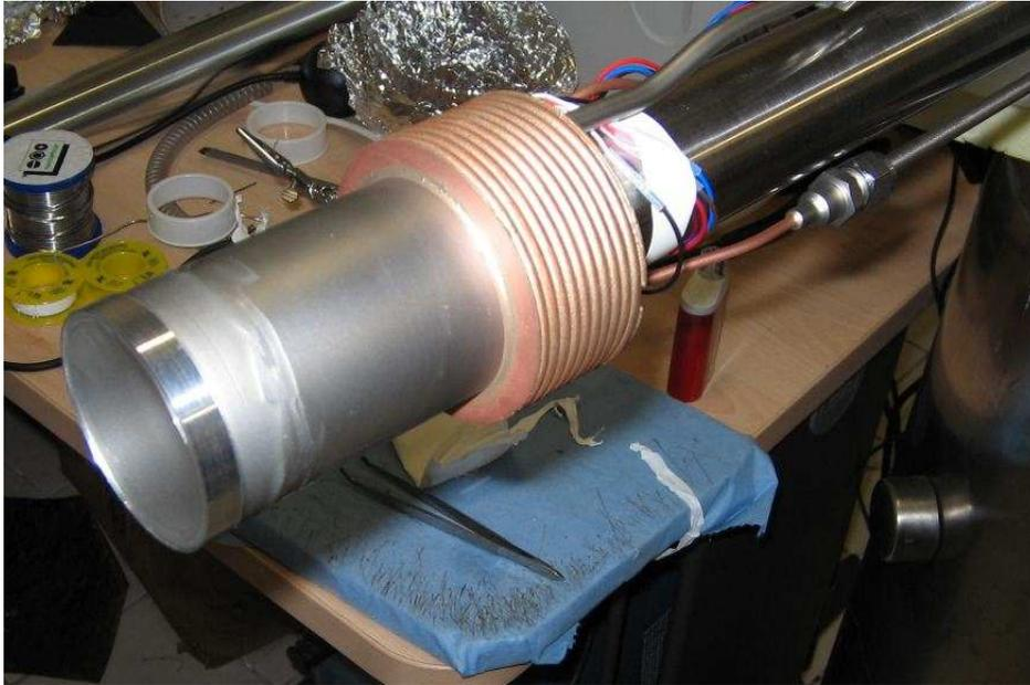
Figure 4.31: A photograph of the liquid hydrogen target used with the  $\pi^-$  beam.
