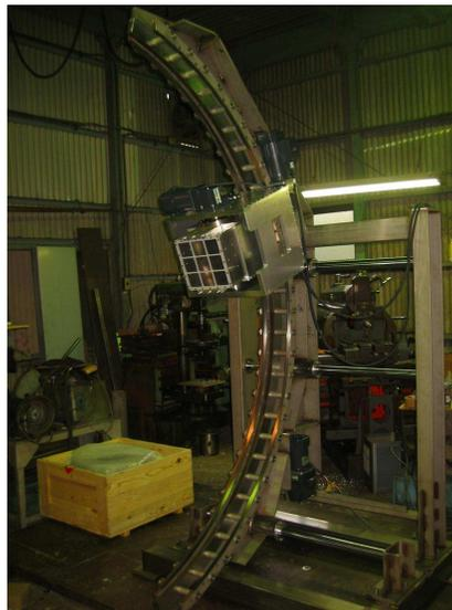
(b) The movable platform for positioning the NaI calorimeter.
