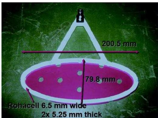
Figure 4.6: A photograph of the muon stopping target labeled with dimensions.
