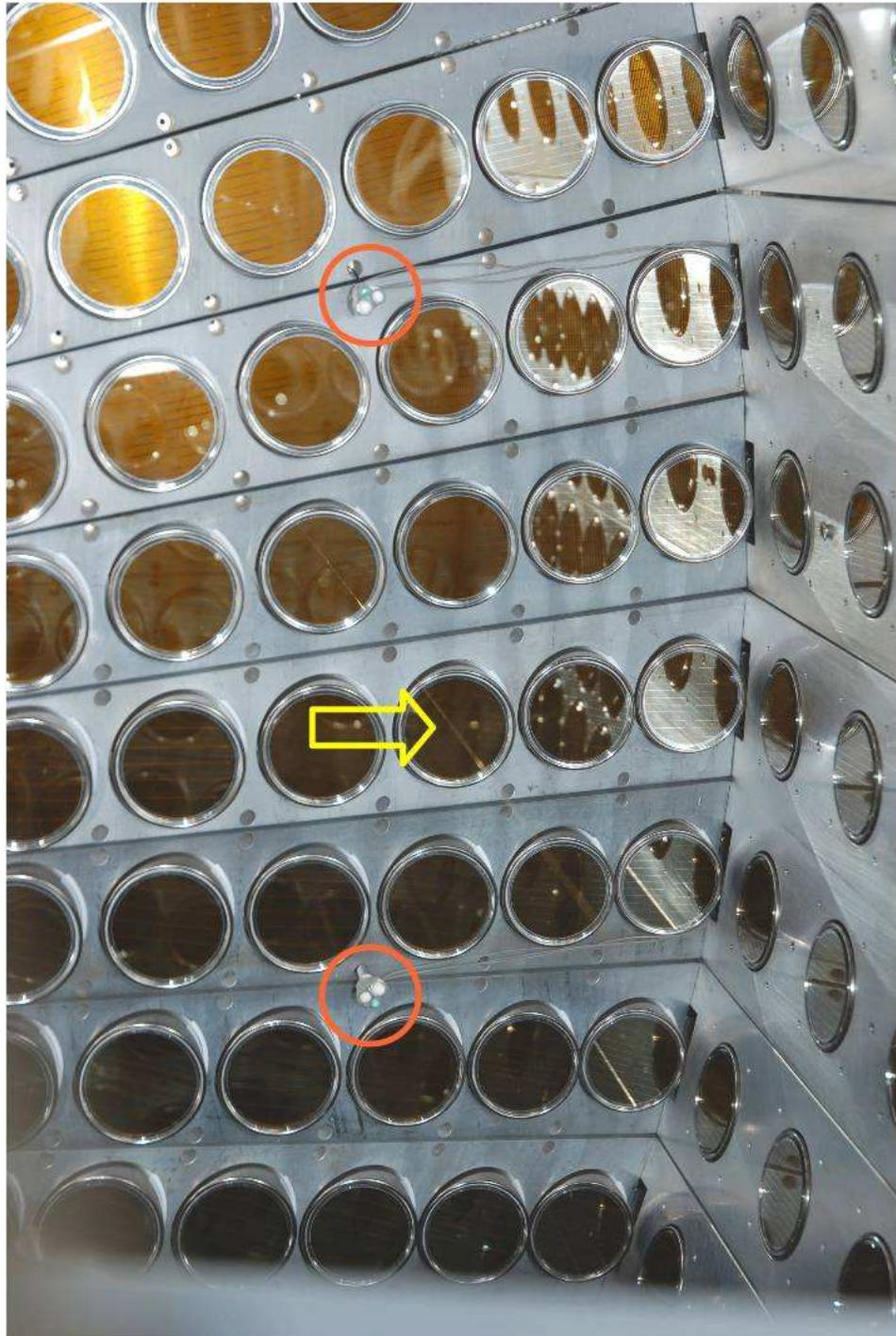
Figure 4.25: A photograph of the mounted LED and alpha sources. The orange circle indicates a LED and the yellow arrow indicates an alpha source wire.
