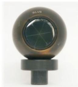
Figure 5.7: Photograph of the corner cube reflector which was used by the PSI Survey Group for the optical survey 2008 (picture originates from [24]).
