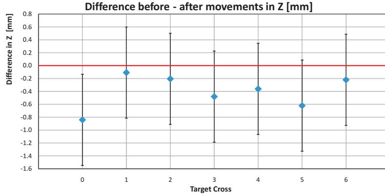
Figure 9.6: Diagram with shown differences between target cross  $z$  coordinates before and after target movements.
