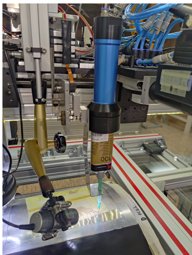
(a) The glue dispenser mounted on the wiring machine.
