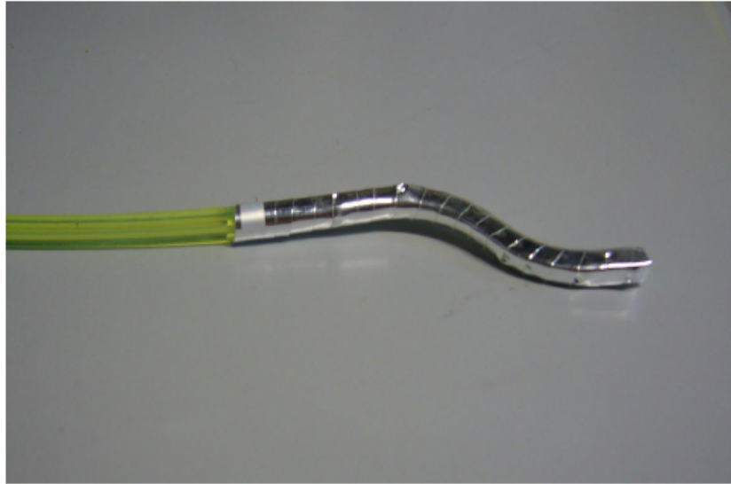
Figure 4.15: Details of the scintillating fiber with covered surface.
