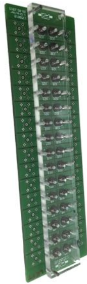
a) PCB with plexiglass alignment mask mounted
