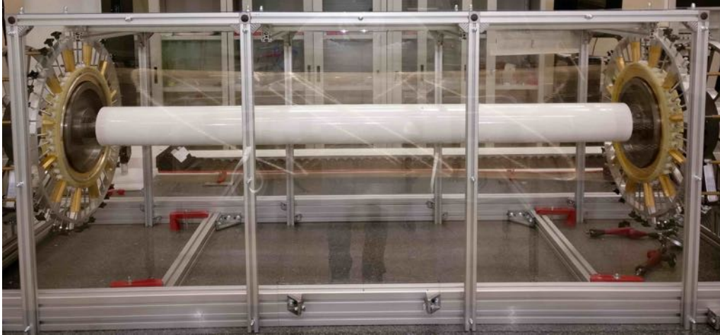
Figure 4.12: The MEG II cylindrical drift chamber under construction.
