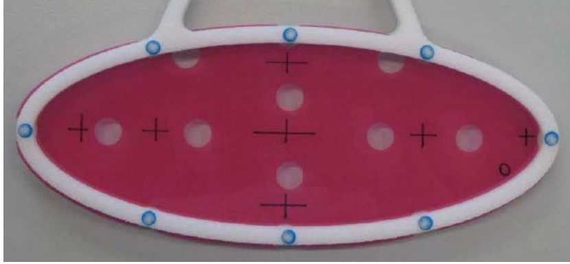
Figure 4.3: The MEG muon stopping target, made of polyethylene and polyester. The crosses and holes are used for alignment purposes.
