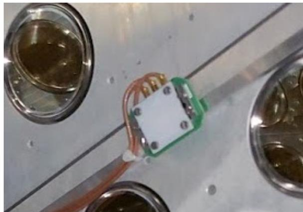
Figure 2.33: A unit of the LED system for MPPC calibration. Three LEDs are mounted to each PCB and dimmed by Teflon.
